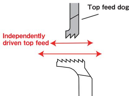
**01** This mechanism prevents the seam from jamming on cross seam sections and eliminates skip stitching.
