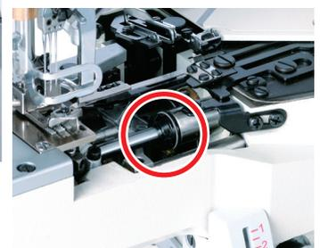
※ Looper shaft can be equipped with only for WT600P series.
