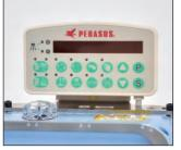
Equipped with the operation panel type controller. Frequently used functions, such as setting machine speed and/or the number of stitches can be called up immediately and set them easily. The sewing machine can be stopped automatically.
