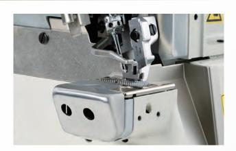
Thanks to the independently driven top feed mechanism, feeding efficiency has been increased dramatically. This feature responds to a wide variety of fabrics, including light to heavy weight fabrics.
