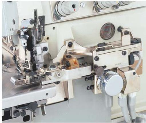
This guide automatically slides as soon as the sensor detects the cross seam section. This feature prevents misalignment due to stitch skipping or plyshifting on the cross seam sections, which tends to occur in blindstitch hemming operations. This device allows the operator to concentrate on the sewing operation.
